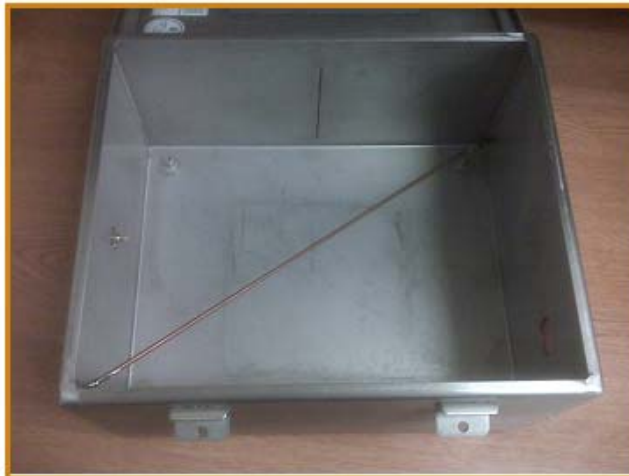
Fig 1c – Inside view showing probe element
