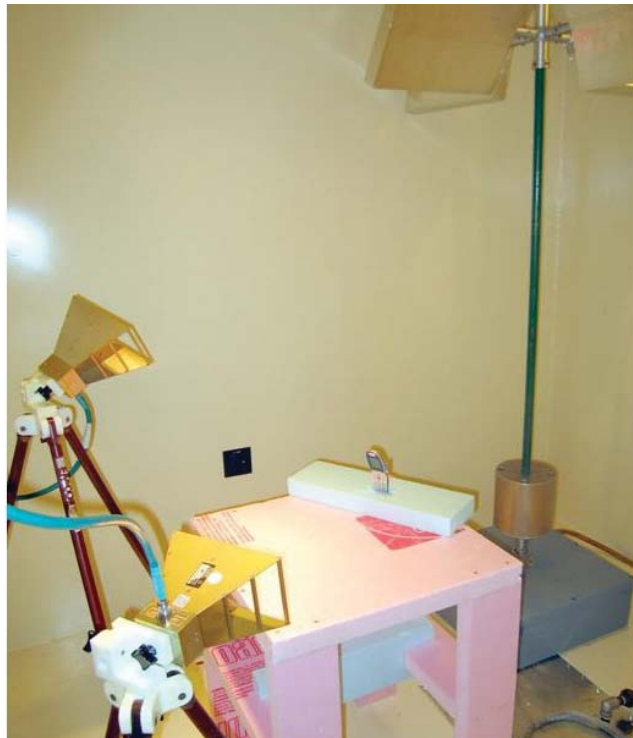
Figure 4. A sample set up in a small test chamber. The front antenna was for communicating with the phone under test.
