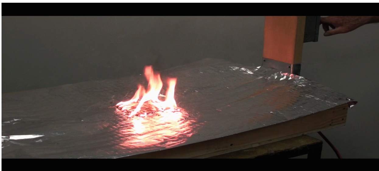
PHOTO #1 (from a previous study) Radiant Barrier Material in Flames After Being Energized by a 20 Amp Circuit
